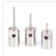
PicoVACQ 1Tc with different probes
